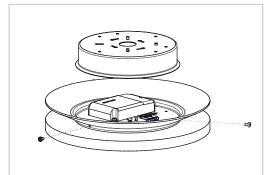
1. Unpack luminaire and remove ceiling plate by removing the three side screws.
