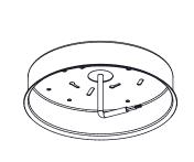
3. Mount ceiling plate on marked positions (make sure electronics can be reached).
