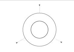
5. Place luminaire careful over base plate and place three screws by hand.
