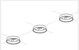
2. Align ceiling plates onto ceiling or wall and mark desired mounting positions.
